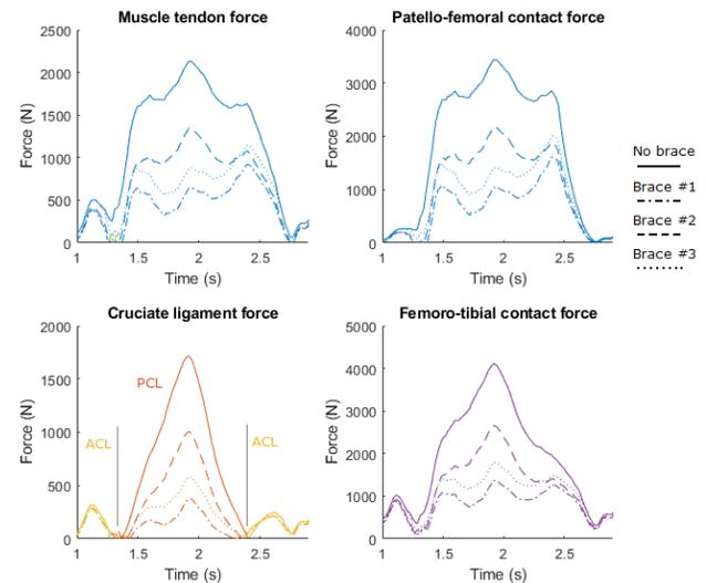
Figure 2: Knee joint loads during a deep-knee bend test with simulated solutions for three different brace load/angle relationships.
