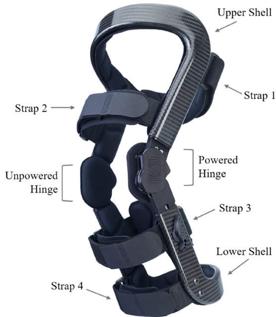
Fig. 2 Schematic diagram of the TCU brace. Components include straps 1–4, powered and unpowered hinge, and upper and lower carbon-fiber shells.
